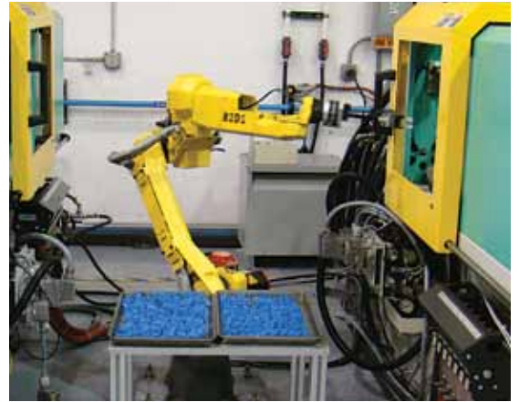
A robot, named R2D1, removes silicone parts from machines in a manufacturing cell at Dynamax's Mundelein facility.
