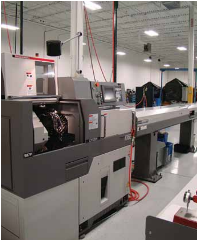
Dynomax recently purchased several Swiss-style machines, such as this one equipped with a bar loader, to help meet the growing demand for medical parts.
